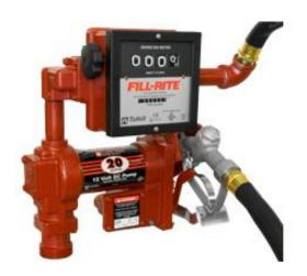
Contractor-grade, industry-standard Fill-Rite pump has an explosion-proof motor with permanent magnet. Steel suction pipe telescopes from 22 in. to 40 in. Features built-in check valve and strainer, hose with static ground wire and thermal overload protection. Comes complete with a 901 Meter and Manual Nozzle. Padlockable. UL listed. U.S.A.
