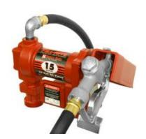
This industry standard DC pump dispenses up to 15 GPM (57 LPM). The FR1210C is ideal for pumping gas, diesel fuel and kerosene. With an amp draw that's easy on your DC power source. Explosion-proof UL/cUL listed 1/4 HP motor. The FR1210C comes complete with 12' static wire hose and manual nozzle.
