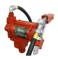
High Flow AC Utility Rotary Vane Pumps Series 300 with a flow rate few pumps can match, this pump provides long life. Explosion-proof UL listed dual voltage 3/4 HP motor (115 and 230 VAC) Motor has sealed bearings, heavy-duty switch and thermal overload protection, built-in junction box, cast iron pump housing with iron rotor and carbon vanes, check valve, pressure relief valve and strainer assembly, Automatic bypass valve, 2" threaded bung for tank openings. 1" Manual Nozzle. 2 Year Warranty.
