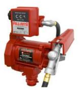
This rugged, positive displacement, heavy duty pump is UL listed. Explosion proof UL listed 1/3 HP motor (115 VAC-60Hz) with sealed bearings, heavy duty switch, thermal overload protection and junction box. Carbon vanes and ceramic/carbon seals reduce wear and repair expense. Integral check valve with pressure relief on outlet side reduces pressure drop and improves vertical lift. Easy removable strainer, automatic bypass valve, 2" threaded bung for tank openings.
