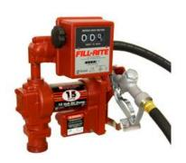
This industry standard DC pump dispenses up to 15 GPM (57 LPM). The FR1211C is ideal for pumping gas, diesel fuel and kerosene. With an amp draw that's easy on your DC power source. Explosion-proof UL/cUL listed 1/4 HP motor. The FR1211C comes complete with an 807C meter, 12' static wire hose and manual nozzle.
