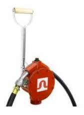
Fill-Rite Piston Pumps have an aluminum body with a stainless steel liner. Providing smooth, continuous transfer of medium viscosity liquids, as well as oil, gasoline and diesel fuel. Pump easily mounts to a standard drum with 2" NPT threaded tank adaptor. 20 gallons per 100 strokes. Made in the USA
