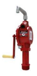
Cast aluminum Fill-Rite pump provides smooth, continuous transfer of medium viscosity liquids, as well as oil, gasoline and diesel fuel. Improved seal keeps water out. Built-in check valve and strainer. Pump easily mounts to a standard drum with 2 in. NPT. Anti-siphoning device, hose with static wire and a 22 in. to 40 in. telescoping suction pipe. Padlockable pump can be set up for reverse flow and is adaptable for drums, kegs or storage tanks. U.S.A.
