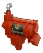
High Flow AC Utility Rotary Vane Pumps. The 313V has an open flow rate of 20 GPM. This pump provides long life. Explosion-proof UL listed dual voltage 3/4 HP motor (115 and 230 VAC) Motor has sealed bearings, heavy-duty switch and thermal overload protection, built-in junction box, cast iron pump housing with iron rotor and carbon vanes, check valve, pressure relief valve and strainer assembly. Automatic bypass valve, 2" threaded bung for tank openings. 2 Year Warranty.
