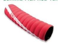
A world-class hose for tank truck, in-plant and oilfield loading operations requiring a strong yet flexible hose. Red cover for easy identification. Exceptional flexibility (one-to-one ratio) for ease of handling. Available in 1 ½"-4". Available in Red or Black.
