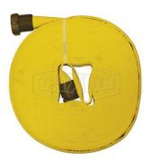
Single jacket all polyester. Tube construction thermoplastic. Rated 270PSI working pressure. Available in 1" and  $1\,\%$ " IDs. Available in 50 ft. and 100 ft. lengths.
