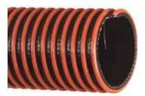
Features: Static grounding wire, 50% lighter than conventional rubber hose, external helix provides for easy drag, and rated for up to 40% aromatic content. Max PSI 65. Available 2"-4"
