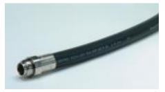
Pumpflex I is designed for curb pump self-service stations and highly sensitive electronic fuel pumps. Pumpflex I is the longest lasting automotive refueling hose in use at service stations today. The durable construction of this hose resists deterioration from fuel in the tube. Available in 5/8", 3/4", and 1". Standard lengths and also on reels. Cut and coupled to customer's specifications.
