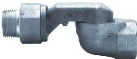
The OPW 241TPS Series of swivels are designed and rigorously tested for applications where easy nozzle and hose handling is important for customer convenience. Swivels are installed in between the nozzle and the hose to provide flexibility in the system to reduce customer strain, position the nozzle properly, and reduce premature hose wear.
