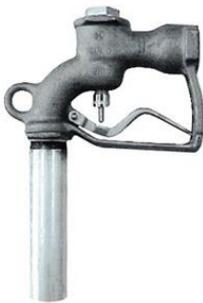
Right angle design, dual poppets, replaceable hold-open rack, dash pot to minimize line shock. Available in 1-1/4" & 1-1/2" threaded inlets.
