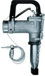
Manual nozzle used for overwing aircraft service. Available with standard 100 mesh strainer and grounding clamp and cable. Available in 1", 1 ¼" and 1 ½" with various spout configurations.
