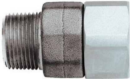
Designed for use with fuel oil nozzles (at inlet only), the OPW 36S provides 360° swivel action. The full-circle swivel reduces the physical strain of aligning the nozzle with the fill pipe. Available in ¾" and 1".
