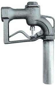
For high-flow, bulk fuel oil delivery service. Designed to handle high flow when line pressure is not a critical consideration or otherwise absorbed.
