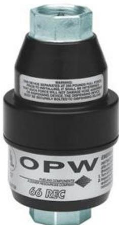
The OPW 66REC is the first dry reconnectable breakaway for the conventional dispensing market. It is designed to be installed on fuel dispensing hoses, and will separate when subjected to a designated pull force. The dual valves seat automatically, stopping the flow of fuel and limiting any fuel spillage, while protecting the dispensing equipment. When reconnecting the separated halves, the 66REC seals tightly on an O-ring before the poppet stems engage to open the valve.
