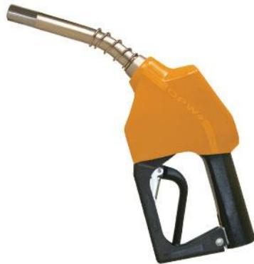
The OPW 11B® Series is designed for use in retail and commercial filling applications including prepay, self and full service, credit/debit card readers or card-lock systems to help prevent gasoline spills. The OPW 11B® will not open until the pumping system is pressurized, and closes automatically when the pressure is removed.
