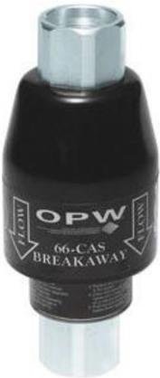
The OPW 66CAS Dual Poppeted, Dry Reconnect Inverted Breakaway is designed to close off the liquid path and the vapor path in the event of a driveaway. Engineered to separate at maximum of 300 pounds of axial pull force, the OPW 66CAS Breakaway will withstand line shocks up to 250 PSI disconnect force, while protecting your dispensing system from catastrophic damage. The OPW 66CAS is developed for use with inverted coaxial metric hoses and designed to meet today's demanding standards.
