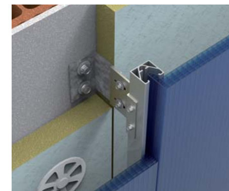
JUNCTION PROFILE DETAIL The interlocking of the panels arcoPlus®626 with the aluminum profile
