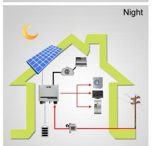
If the battery capacity is insufficient to meet the self-consumption requirements, electricity is then imported from the power grid for use.
