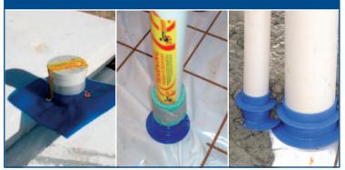
**HomeGuard Collars** are an innovative pre-formed method for protecting service penetrations through a concrete slab. Manufactured in Australia from ridge moulded blue polymer extruded to contain Biflex Termiticide (HomeGuard Collars are the only moulded collar on the market that contains the power of a termiticide).
